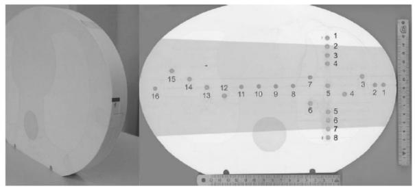
Fig 1.: Right image: Distribution of the TLD measurement points on one phantom slice. 16 points allow measuring a "depth dose" curve, 8 points lie on a "profile" of the 20 cm x 10 cm field. The primary irradiation area is pointed out with a changed background. Left image: the TLD slice is sealed with a further slice. Both slices form the "TLD sandwich".
