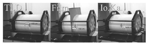
Fig 2.: measurements with TLD, film and ionisation chamber
