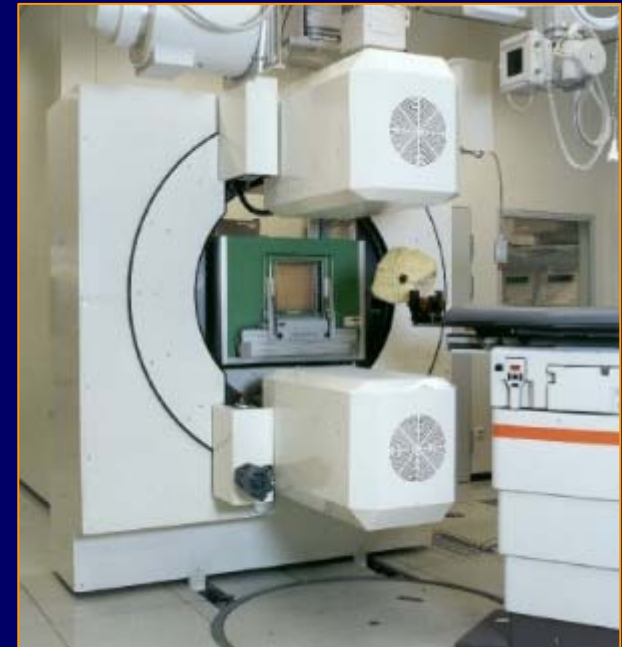
Double head positron camera developed by FZD at the treatment site of GSI Darmstadt.
