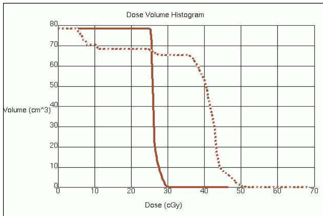
Fig. 6: Cumulative DVH for the rectum with daily CBCT (solid) and daily MVCT
