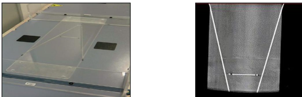
Fig. 1: PMMA frame used in immobilisation and for image registration (left) and its T2 image (right).
