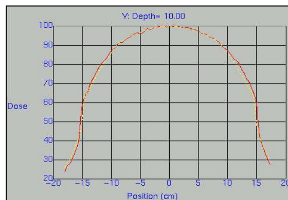
Fig. 2: Measured and calculated Inplane Profile for the CBCT dose calculation model
