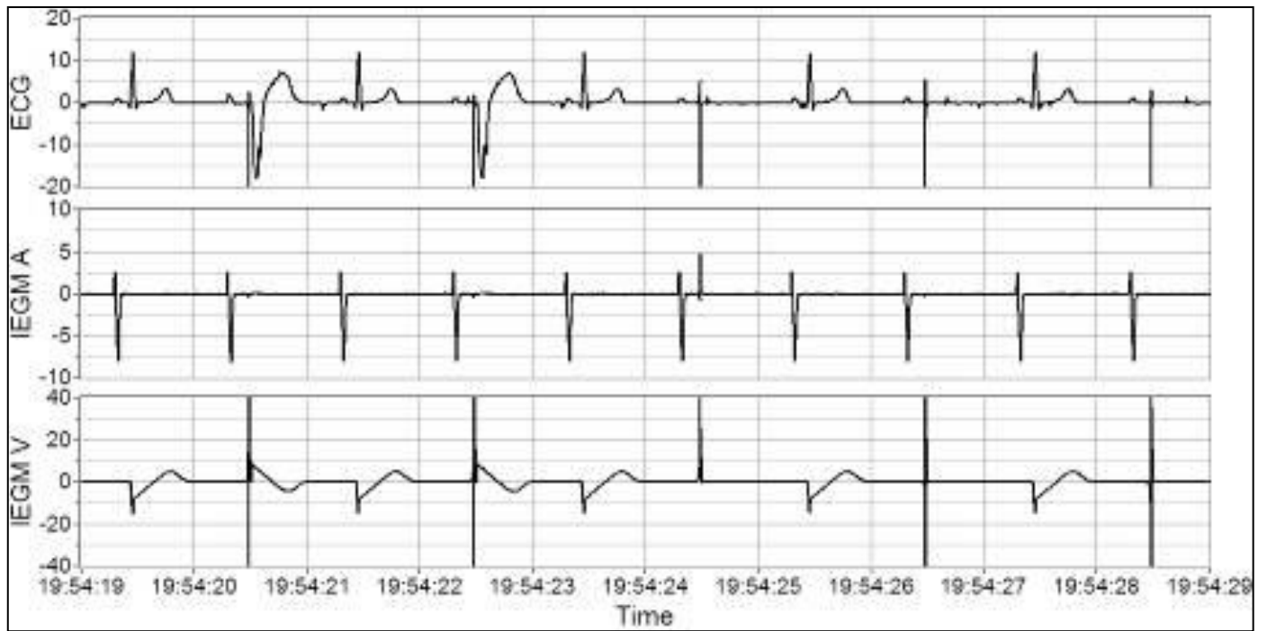
Fig. 2: Pacemaker operation showing stimulation failure (starting at 19:54:24) after exposure to 135 Gy / 18 MV.
