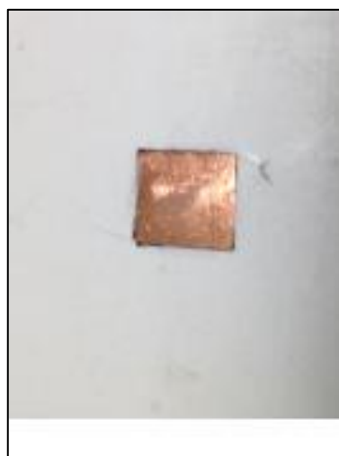
Fig. 1: A copper slab of dimensions 1.0 \times 8.0 \times 8.8\text{mm}^3 embedded in an adapted RW3 slab for measurements within the Octavius 4D phantom.
