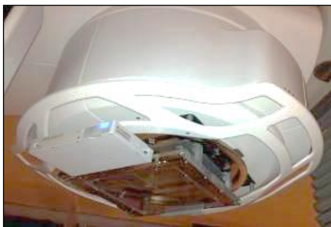
Fig. 1 . The DAVID chamber attached to the Elekta Synergy linac
