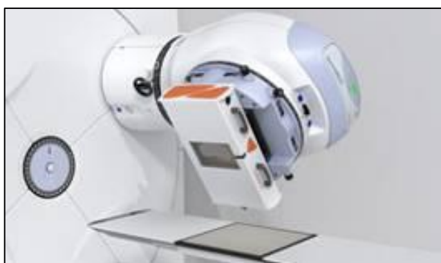
Fig. 1: CobraLeaf mounted on a Best Theratronics Gammabeam 100-80 (Phoenix) Co-60 treatment device
