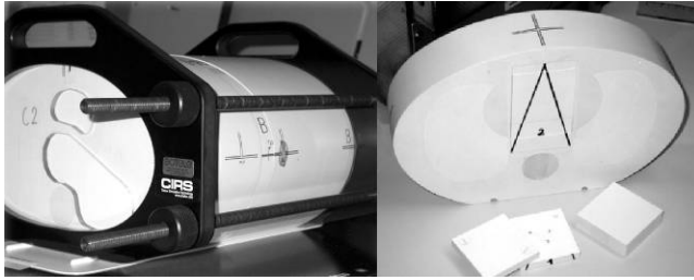
Fig. 2 Left: CIRS Thorax phantom with Perspex structure slices. Right: „mini phantom“, dedicated to check the absolute calibration
