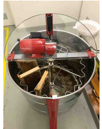
The honey extractor : using centrifugal force, the honey is extracted from the frames
